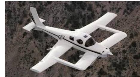
The canard design is inherently not a platform for short fields, so the Grizzly was an airframe to test what the limits were of the canard layout in the STOL mission.
