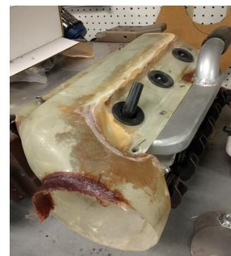
plenums being configured instead. I wanted my plugs accessible and a plenum cooling system. LS1 boots will allow me to route external plug wires.
