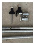
jig that will enable you to accurately measure over and around obstructions. I built mine with removable ends so that I can replace the center section with longer or shorter lengths to better suit my needs. I have 4', 6', and 10' center sections for my trammel jig to square up the wing spars for various airplane projects. Fortunately, EMT conduit is cheap.
