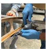
fillet, install the rib locating jig, check that the ribs are plumb, and finally re-fit the drag tubes. Wait 24 hours for curing. So far, we completed 4 ribs. We will complete the last 5 at the next workshop and finally rinse and repeat for the 2<sup>nd</sup>
