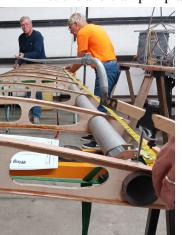
Using the ½" couplings, attach each end of your jig to the long, straight center section of ½" EMT.
