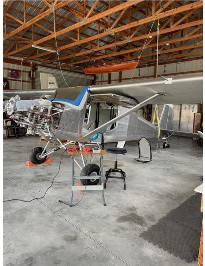
Now he is hooking everything up to the system and to the Engine Control Unit. He has installed the Dave Fife hoerner type wing tips and tail caps. The wing tips will decrease the stall speed and improve low speed handling of the aircraft.
