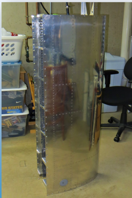
Removable Wet Wing Fuel Tank
