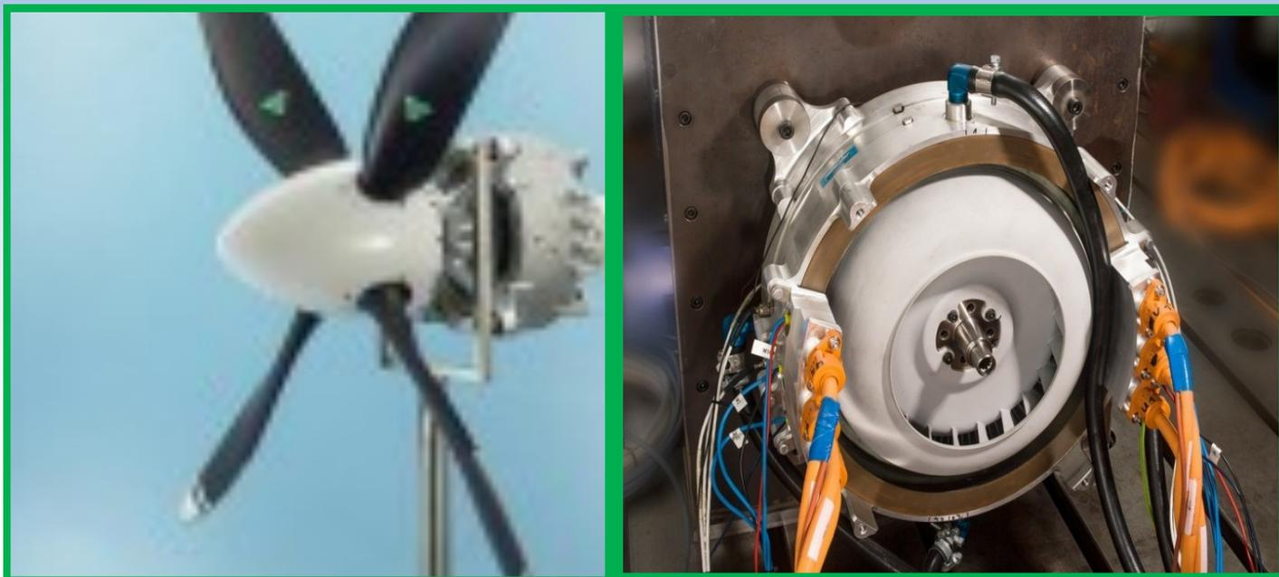
Researchers at Siemens have created a new prototype electric motor specifically designed for aircraft that weighs in at just 50 kg (110 lb) and is claimed to produce about 260 kW (348 hp) at just 2,500 RPM. With a quoted power five times greater than any comparable power plant, the new motor promises enough grunt to get aircraft with take-off weights of up to 1,800 kg (2 ton) off the ground.
