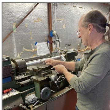
Robert Skalany puts his talent and lathe to work to solve a problem of powder coating that is too thick on a pair of steel flap torque tubes.
