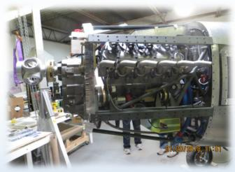
New Corvette 7 liter V8 \$5,500 from PC performance, water cooled, non turbo
