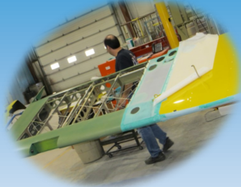
Repairing wing Covering
