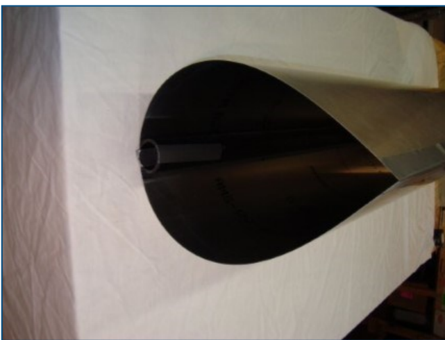
PVC or metal pipe sets the final bend radius
