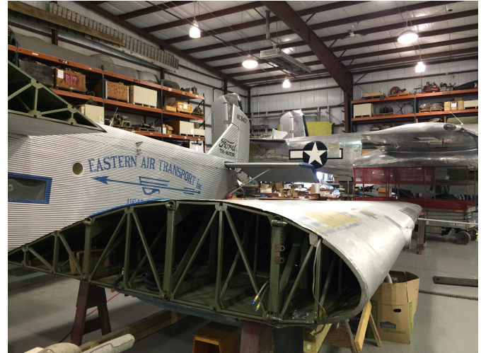
(Photo: John Salz) 4AT in for maintenance. John points out the "bridgelike" truss structure in the wing of the Ford.
