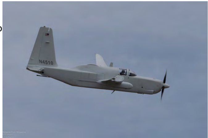
Grob Egret in flight, a German design that was to be their Cold War recon aircraft similar to the American U-2. This aircraft is now a "high altitude towplane" for the Perlan glider below. (Photo by Chris Bildilli)
