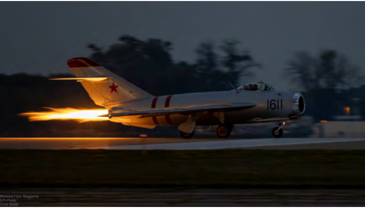
The MiG-17 with full afterburner on an evening departure. The unique afterburner on the MiG more closely resembles an F-111 fuel dump as the flame doesn't look focused as most afterburning engines. It's quite visible during the day as well. (Photo Chris Bildilli)
