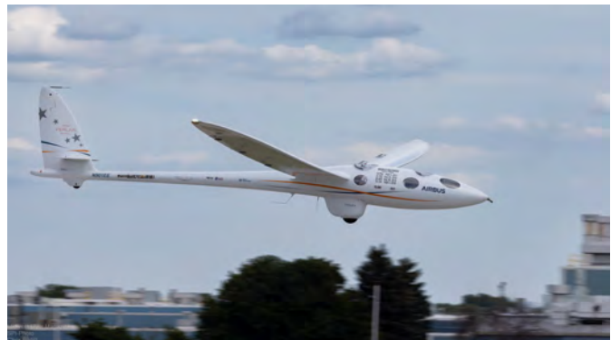
Airbus Perlan high altitude research glider which cruises normally at 50,000ft but can operate at up to 90,000ft. (Photo by Chris Bildilli)
