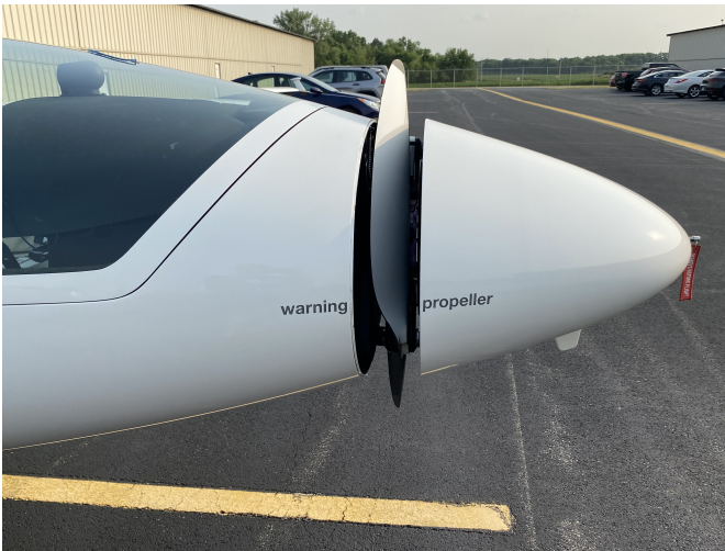
Does a retractable prop make it complex? After a powered takeoff and climb, the propeller folds up and the nose cone closes improving the aerodynamics as it soars)
