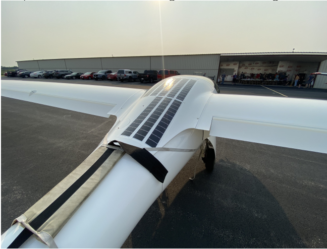
(the solar panels assisted a battery located in the tailplane that gives power to the aircraft's electrical system)
