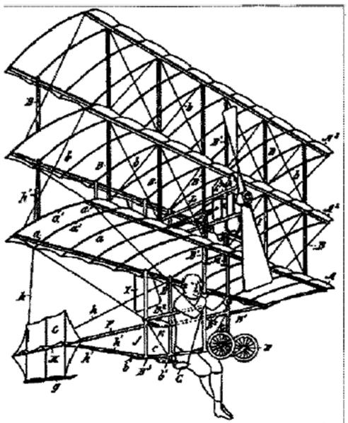
This is an illustration from a British patent application filed jointly by Octave Chanute, Chicago, and Augustus Herring, Sr. Joseph, Michigan, in 1896 for a heavier-than-ait flying machine. A rather primitive design that used weight-shifting for control, it was based on the Chanute-Herring triplane glidez flown by Herring in the summer of 1895. The patent, No. 15,221, was issued in June 1897. See page 11 for more information.
