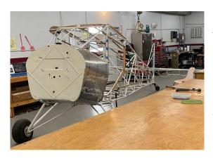
For those that haven't heard, we have restarted the TaylorCraft project. We are currently moving forward on the fuselage with lots of work to do. We have control cables to make and install, all new pulleys to install. We also need to run wiring for lights and such, plus build out the luggage compartment, refinishing the doors, etc. As you can see, we are working hard to get more organized and get moving forward in a manner more like kit planes are built. Once the
