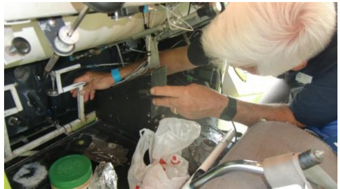
George Bedeian is helping the owner put pressure on the brakes so they can properly bleed. Image Courtesy of Adam Santic, EAR Volunteer and Newsletter Editor-in-Chief.
