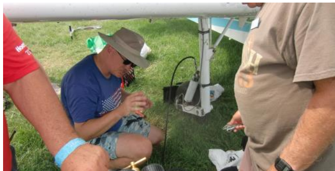
This 1982 LA-4-200EP "Lake EP" needed its struts to receive nitrogen. Image Courtesy of Adam Santic, EAR Volunteer and Newsletter Editor-in-Chief.
