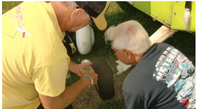
George Bedeian (right) helping the owner of a Wittman Tailwind with his brakes that needs bleeding. Image Courtesy of Adam Santic, EAR Volunteer and Newsletter Editor-in-Chief.
