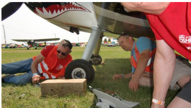
John Ruyle and Allen Numerick helping raise a 2008 Van's RV-8 with an axle block.
