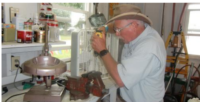
George Bedeian (left) and an unidentified person working on a cowling latch project. The unidentified person is now drilling a hole for the latch.
