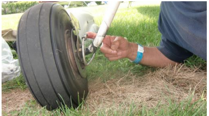
George Bedeian plugs up the hole to a Wittman Tailwind with his finger to keep the brake fluid from leaking out. Image Courtesy of Adam Santic, EAR Volunteer and Newsletter Editor-in-Chief.
