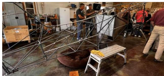
Bob and Penny Johnson's RANS S-20 Raven's fuselage that requires pieces to be welded together.
