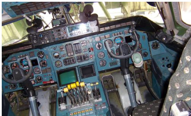
Cockpit controls and ceiling fans. They were using a Garmin GPS III as their primary means of navigation.
