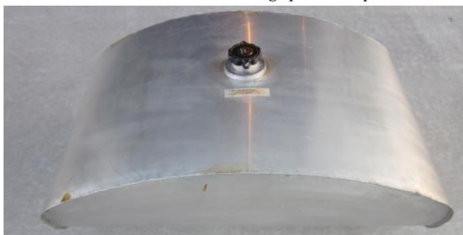
Falconar F-12 Cruiser 23-gallon fuel tank.
