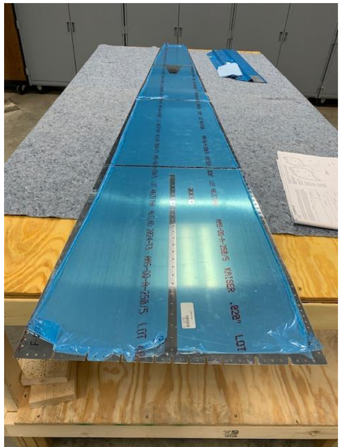
Van's RV12-iS tail cone skins being prepared for assembly.
