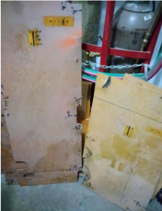
Old floorboards used for patterns.
