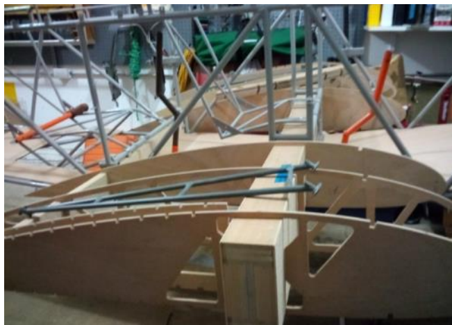
A very rough view of the center section wing ribs in place on the spars.
