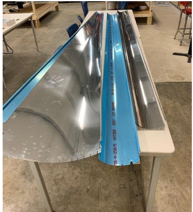
Van's RV12-iS tail cone skins being prepared for assembly
