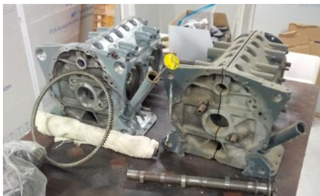
Modified Lycoming O-290-G awaits reassembly, while a possibly "junkie" extra, unmodified casing awaits its own destiny.
