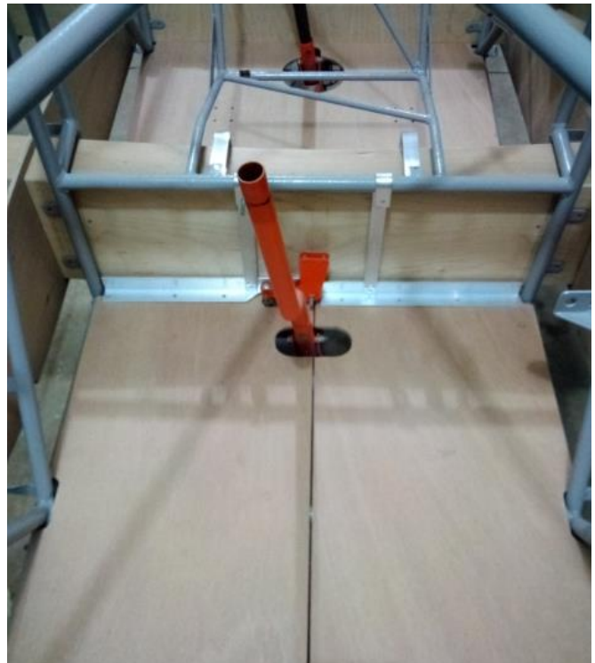
New Okume (Marine) Mahogany floorboards nicely fitted.
