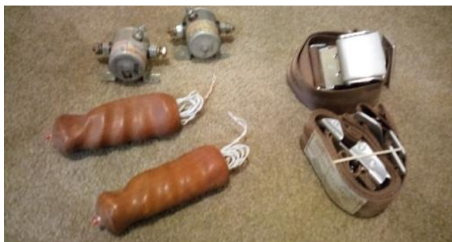
Pair of 24-volt 120-Amp starter or panel relays, pair of walnut contoured wood stick grips, and lap belts.
