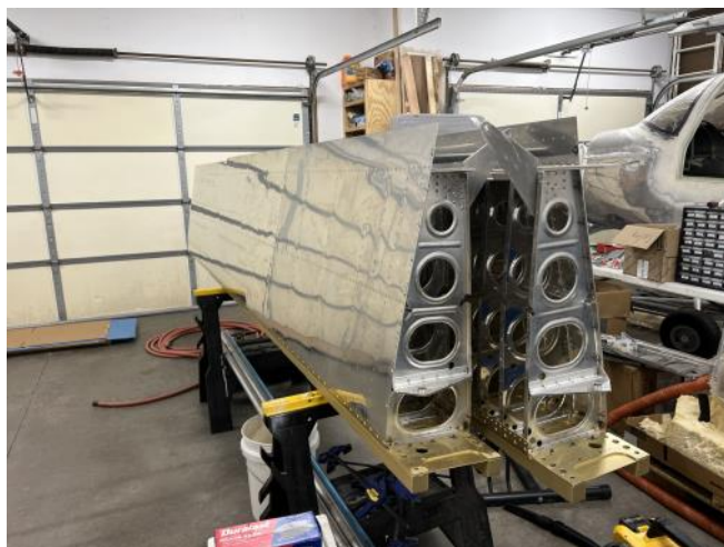
Shown here is the wings in Chris' build shop, also known as the garage, on the wing rack, awaiting attachment to the fuselage.
