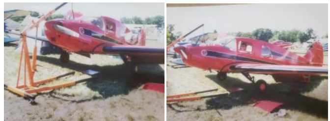
Mark and Judy Ohlinger (as PIC) performing a landing gear check at EAR on their 1946 Bellanca 14-13 Cruisair Senior (N86937).
