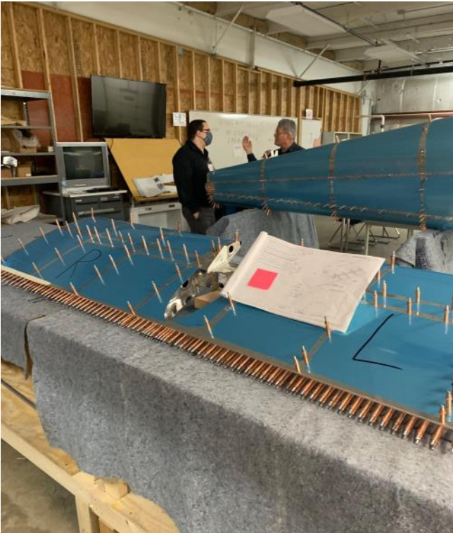
Craig Olson and Zach making progress on the horizontal stabilizer.
