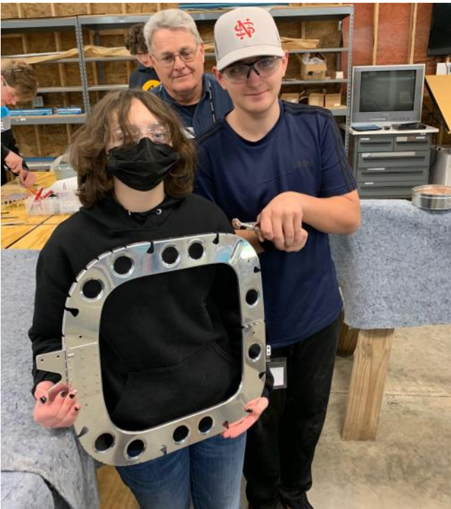
Gabrielle, Denver and Craig Olson are proud of their work on the tailcone bulkhead.
