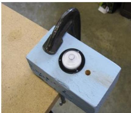
I started with a square block of wood at the drill press, drilling a hole through the block. I then clamped that block of wood to my workbench, placing the second bubble level on the block. If the block is not level it needs to be shimmed to make it so.
