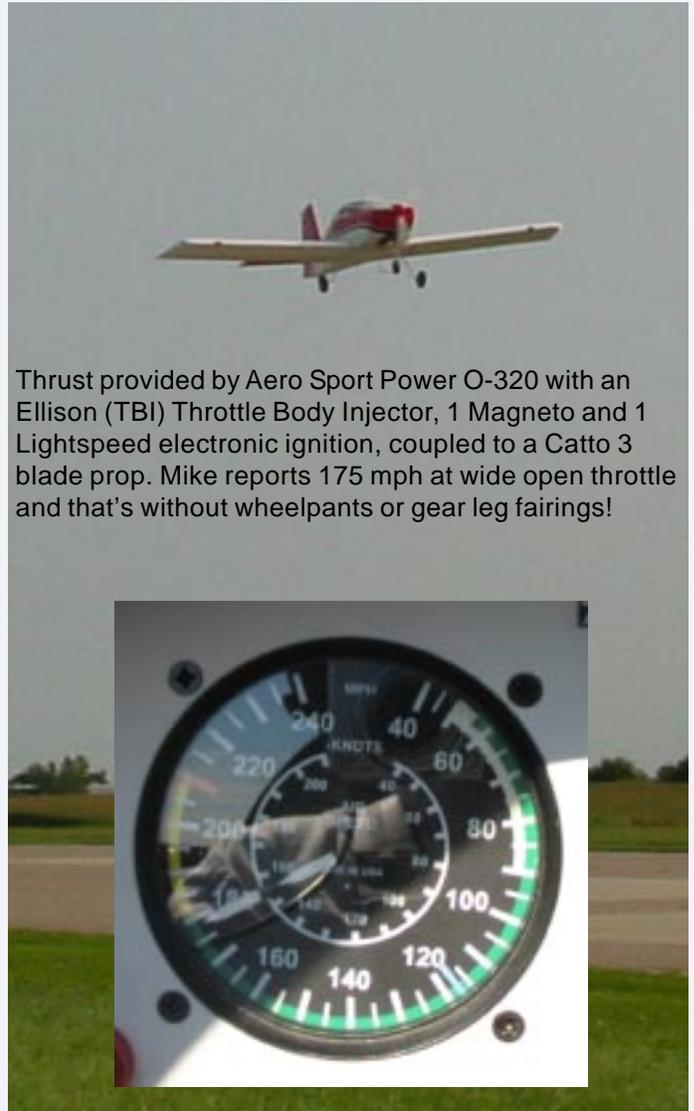
Thrust provided by Aero Sport Power O-320 with an Ellison (TBI) Throttle Body Injector, 1 Magneto and 1 Lightspeed electronic ignition, coupled to a Catto 3 blade prop. Mike reports 175 mph at wide open throttle and that's without wheelpants or gear leg fairings!
