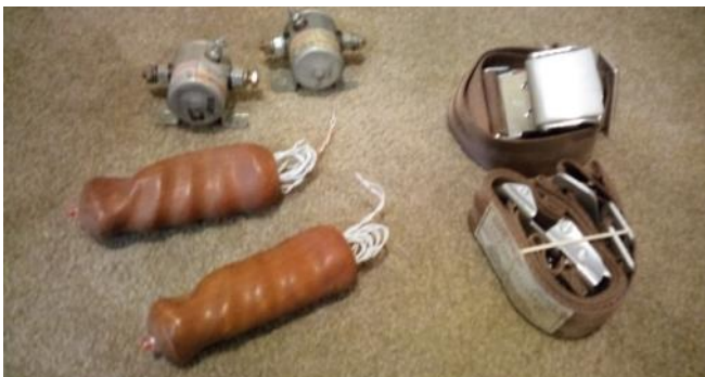
Pair of 24-volt 120-Amp starter or panel relays, pair of walnut contoured wood stick grips, and lap belts.
