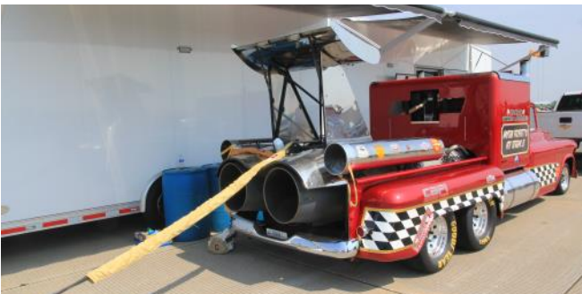
Hayden Proffitt II's highly modified 1957 Chevrolet Pickup Truck with two Westinghouse J34 engines.
