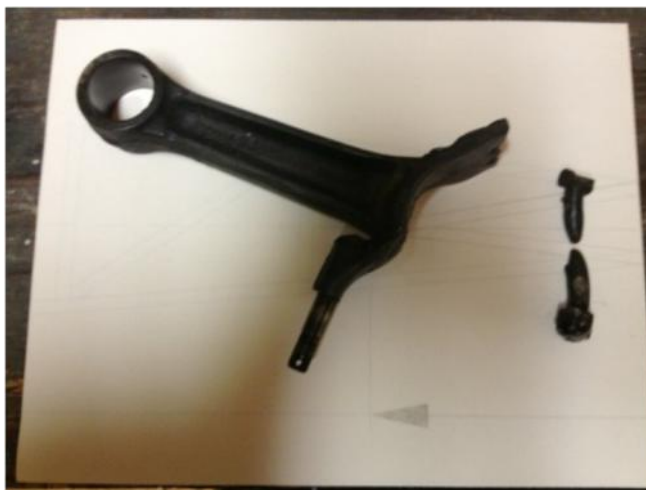
Number two rod and failed bolt with nut still attached
