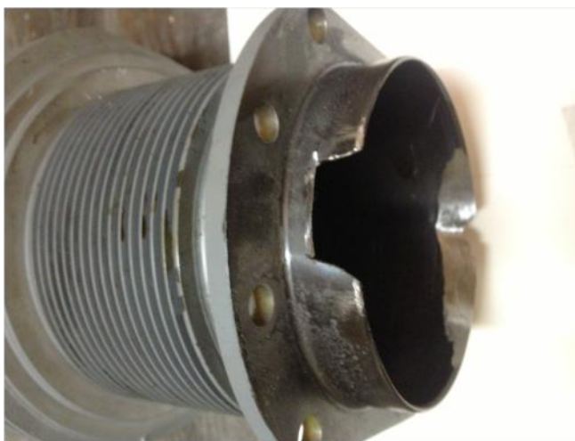
Number two cylinder base after cutting away skirt to release it.
