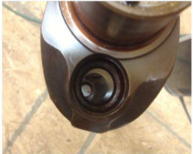
Sludge Tube as Installed in a Rod Journal
