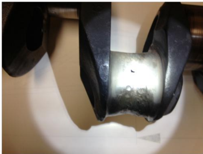
Number two rod journal damage, note the oil relief hole partially closed off
