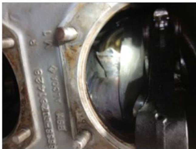
View through the number 1 Cylinder base opening before Disassembly
