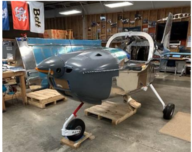
Front view of the Van's RV-12iS with a Rotax 912iS engine and a ground-adjustable Sensenich composite propeller.
