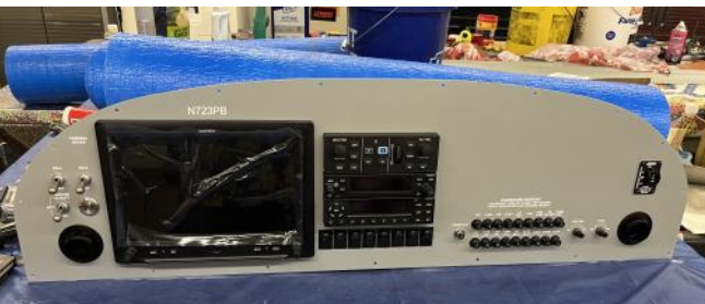
Bob Johnson's RANS S-20 Raven (N723PB) project. This is the panel. Image Courtesy of Bob Johnson.
