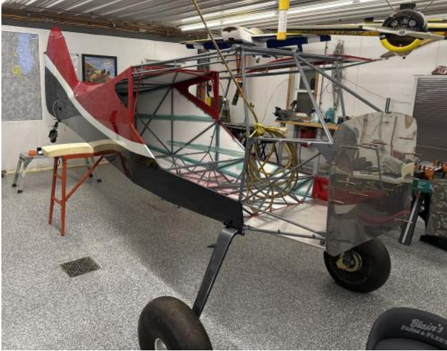
Bob Johnson's RANS S-20 Raven (N723PB) project. This is the fuselage. Image Courtesy of Bob Johnson.
