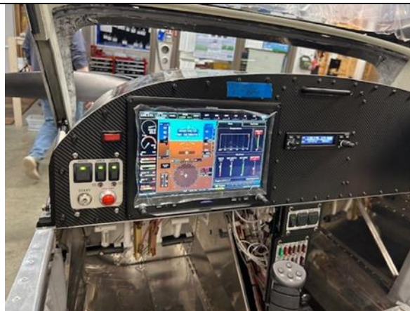
Garmin G3X Touch Display being updated and configured. Image Courtesy of Tom Shelton.
