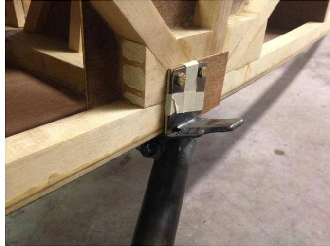
**Fittings attached to fuselage**
