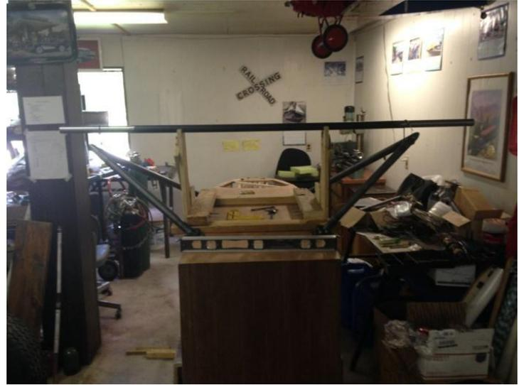
**The weld jig and long pipe used to align the axles to the gear legs for tack welding**
