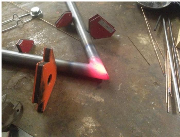
Welding the front and back gear legs together.
