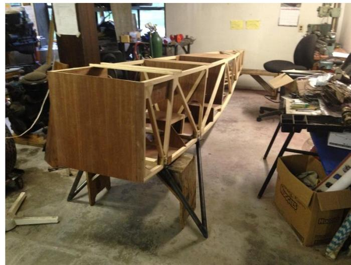
Test fitting the gear legs to fuselage before welding the axles on.
