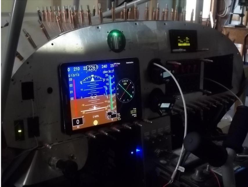
The attached photo, shows the 1st power-up of my (mostly complete) panel. For this test and until I get everything finalized, I am powering the panel from a car battery to avoid draining ships power and generating any Lithium-Ion induced sparks and smoke should something not be just right.
