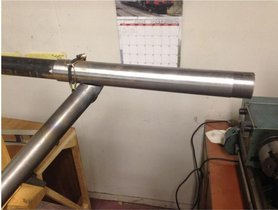
**How the axle fit to the gear leg just prior to tack welding.**
