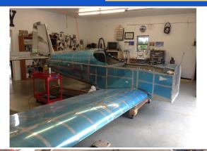
Wings and tail attached. I have recently removed both to allow me easier access to fuselage for building canopy frame, wiring and fuel/brake line plumbing.
