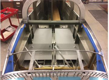
Cabin interior view showing canopy frame which is the structure I am presently working on. My RV-9A will have a tip up canopy. Fabrication of the canopy frame and bubble canopy is a slow, tedious process which is making me balder than I already am.
