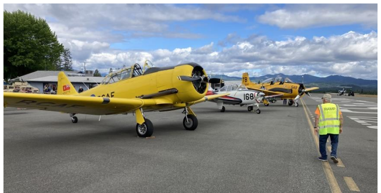
Beautifully maintained examples of past military training aircraft. In the foreground is a WWII vintage Harvard Mk 4. In the middle is a Beech T34 "Mentor" in Navy colors, with a North American T28 "Trojan", also in Navy colors, alongside. Yep, that's Richard Colton walking the "zipper line".
