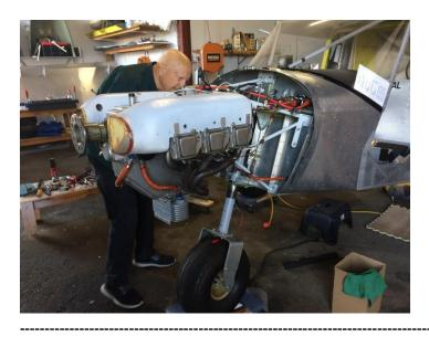
Dick is finishing up his firewall forward tasks. He has the engine controls connected and is routing plumbing lines. Some wiring work is yet to be completed before he can run the engine. He's not making any predictions.
