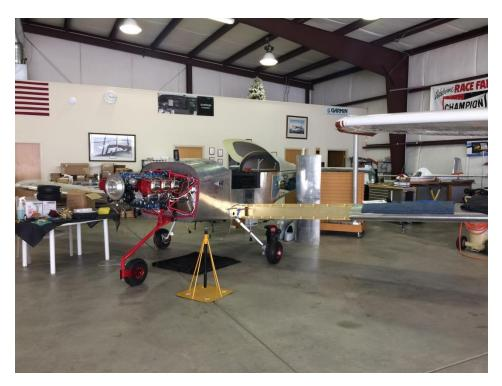
The RV10 builder assist project has sprouted wings and the left wing long range fuel tank was being fitted when I took this photo. Ryan says there's another RV10 project behind this one, but it will be a standard kit. Quick build kit lead times are out into the next millennium. After that it's an Evolution and maybe a Bearhawk, so he figures he's backlogged out to September of next year.
