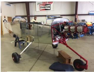
The RV10 project now has a brand new IO540 on the firewall in prep for plumbing and wiring runs. Some wiring in the fuselage is also in place.
