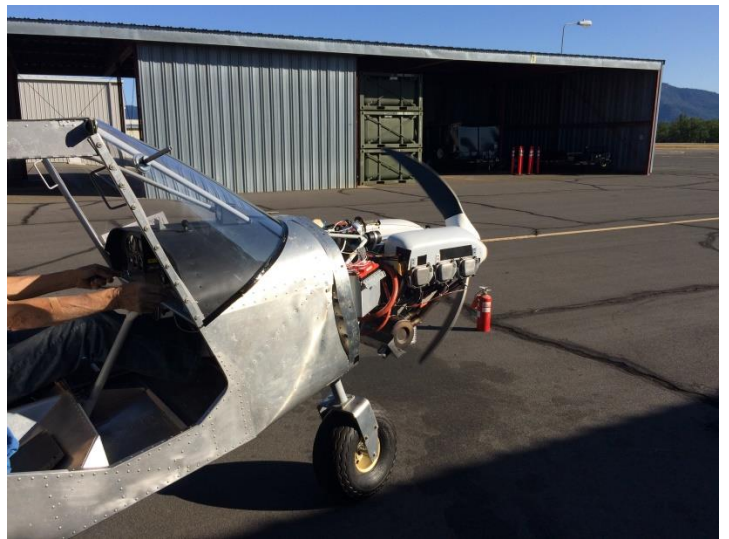
July 17 th -1 st engine start. Unfortunately, there was no opportunity to do normal engine runs as the oil pressure gauge was not reading. Subsequent troubleshooting pointed to a faulty sending unit. A bit of money and time will fix that.
