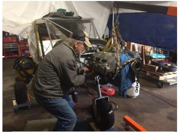
Yes, Dick's engine finally made it back from Tennessee and is now temporarily installed on the front of his CH701. Here, Phil lends a hand installing one of the engine mount bolts. Let the fun begin.
