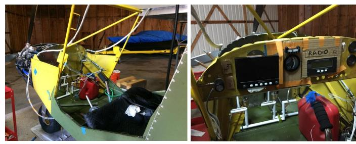
And here is Dennis' 701. The wings are on and control system hook-up is complete. Here he has stripped out the old panel in preparation for installing a new one.
