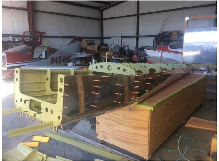
Ryan is assisting Dutch Bros. pilot Drew Meltebeke with his AirCam project. This is the fuselage under construction. A very interesting homebuilt with twin Rotax engines. Sort of looks like a canoe with wings.
