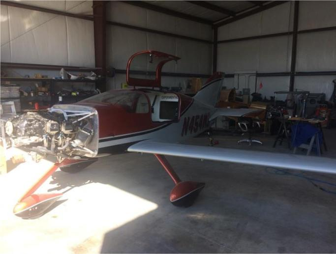
First you buy an airplane, then you take it apart. Dave Palmer's Tango is getting a constant speed prop, a yaw axis autopilot servo, a repair to the elevator trim hinge installation, and a new interior.
