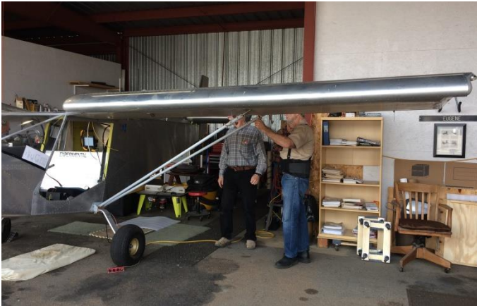
Dennis and Phil complete the wing strut attachment for the left wing. The right wing is already in place.
