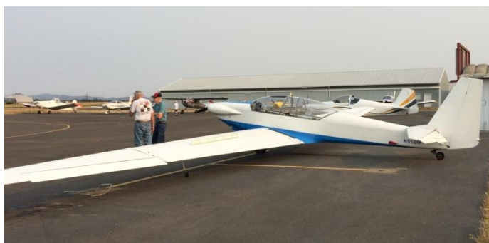
1974 Sportavia RF5B motorglider owned by Collin Gyenes of McMinville. Powered by a Limbach 1700 VW conversion. Used to be one of these at G. P.
