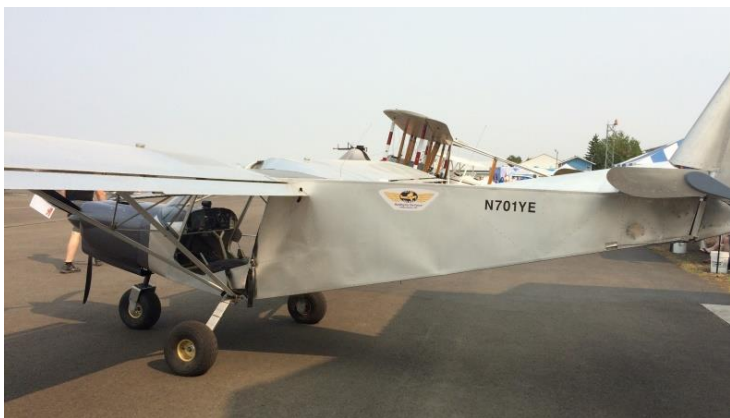
The Chapter's Teen Build CH701, powered by an Aeromomentum AM15. This is a Suzuki-based engine . Bill McLagan was the primary mentor for the teen group builders. The aircraft has completed its flight test program and will soon be Missouri bound.
