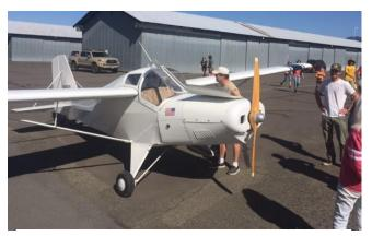
Had to find a way to squeeze this in. JD brought his newly acquired Cygnet homebuilt over so we could all give it a good look. A 2-place shoulder-wing design from the 70's, it's powered by a Revmaster VW conversion
