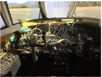
Oh yeah, that's it. N749L is getting a complete avionics swap to install a Garmin system removed from an airplane in Nevada. Man, what a rat's nest. Sure glad I don't have to trace all those wires.
