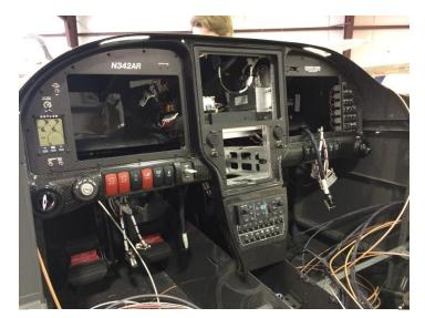
This will be one very well equipped RV10. The new panel is the latest installation and it certainly is impressive. More wiring is being added forward of the firewall. It will even have air conditioning!
