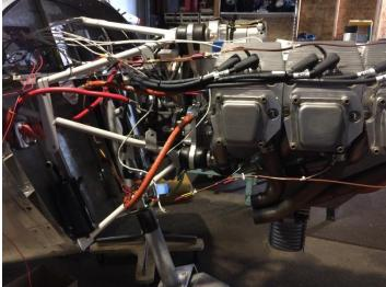
These two photos show Dick's progress on his CH701 wiring installation. Considerable work has been done to complete connections and tidy up the routing. No promises, but he's hoping to report at the next meeting that he's made initial engine runs.
