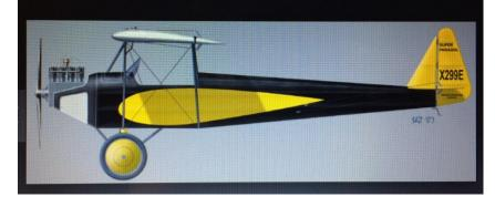
Ed Heath's Parasol first flew in 1926 powered by a 25 hp Heath-Henderson motorcycle engine. Ultimately, it could be purchased factory complete for \$995, assembled from a kit, or built from plans.
