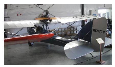
An authentic early 30's Curtiss CW-1 "Junior" on display at WAAAM. Some 270 were produced in 1931 and 1932. It was powered by a 45 hp 3 cylinder Szekely radial engine. The engine had a bad habit of throwing cylinders, thus the cables that can be seen in the photo connecting the cylinder heads. Hmmm, wonder if there was a STC for that.
