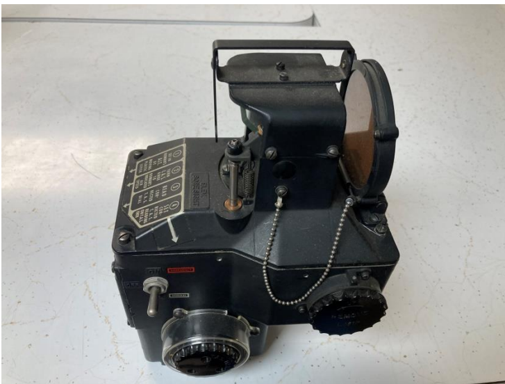
Sperry Gyroscope Co. K13 Compensating Gun Sight. These were installed at the waist gunner positions in both B17's and B24's late in the war.
