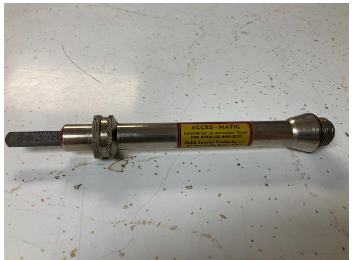
Now this is unique, a cylinder compression tester very much like a tire gauge. Called an Accro-Matic and made by Gabb Special Products, Inc. Used in sets, mostly on radial engines. Install one each cylinder, motor, and viola(!), get the pressure in all cylinders in one shot. We have a set of six.
