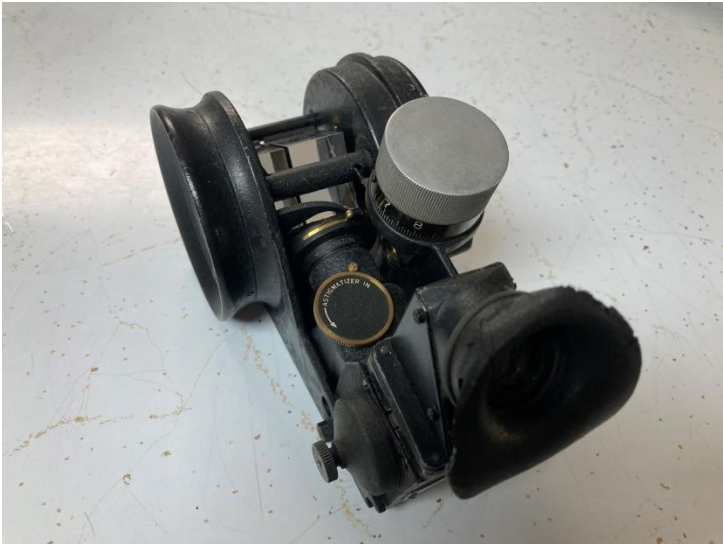
Pioneer Instrument Octant Model A5. In the original case and appears to be complete with manual. There's a Serviceable Part Tag with it dated April 12, 1938.
