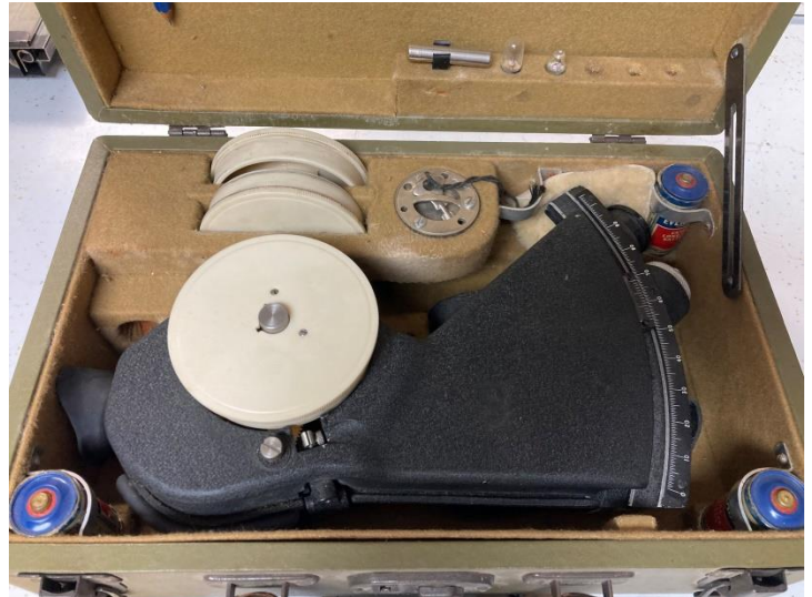
Link Aviation Co. Bubble Sextant Model A12. Looks like there might be some missing accessory pieces, but it's otherwise in good shape and in the original case. The donation record is dated 1991.
