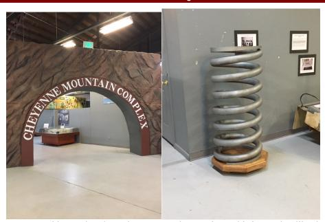
Is this a Colorado Spring or a Manitou Spring? This is a spring like the ones inside Cheyenne Mountain to stabilize the facility in the event of a nuclear attack.
