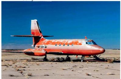
The four engines that mounted on the tail (two on each side) were long since removed.
