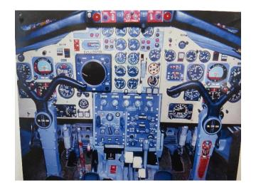
The answer is: The "Parking Brake"...of course used to lock the brakes for parking (after the brakes cool down – if used heavily on landing...which was hardly ever the case). In the picture it is just to the right of the #2 engine throttle.
