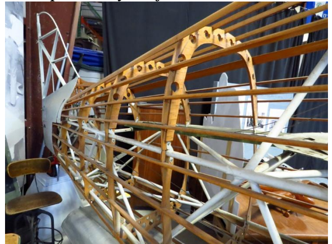
Steel tube fuselage and lotsa' wood! Fabric covered.
