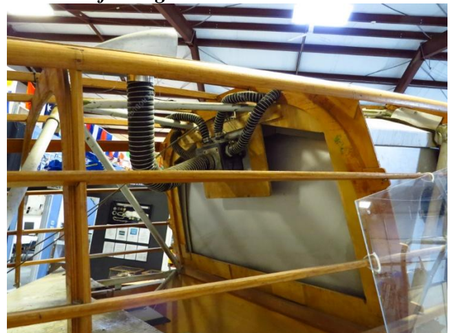
Waco environmental control system – not complicated but very reliable!
