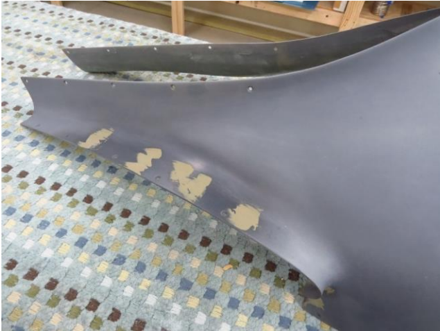
Filling a few minor imperfections in a fiberglass fairing for the vertical and horizontal surfaces.
