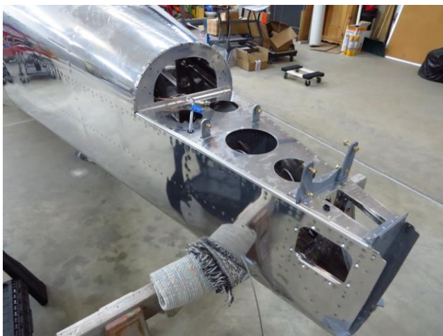
Rear fuselage attachment points for vertical and horizontal surfaces.
