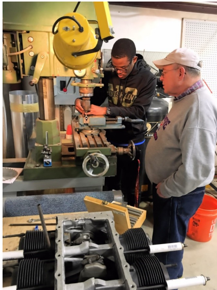
Derrick setting up the milling machine to drill a hole for the cotter pin that will keep the tailwheel assembly for the Piet in place
