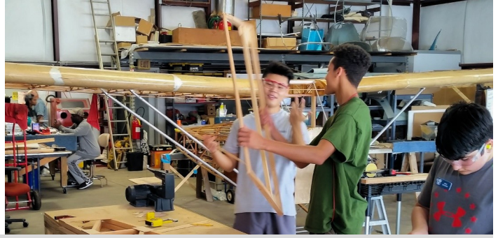
After making all of the ribs for the 2-place Pietenpol it's on to the elevator and rudder surfaces.
