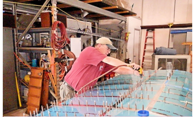
Joel match drilling the wing skins on the left wing prior to closing it up!
