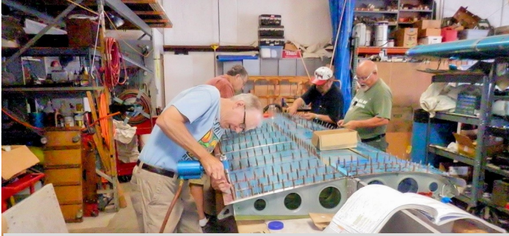
John, Louis, Ron and Keith prepping the left wing prior to riveting the skins. Thank goodness for the pneumatic puller!
