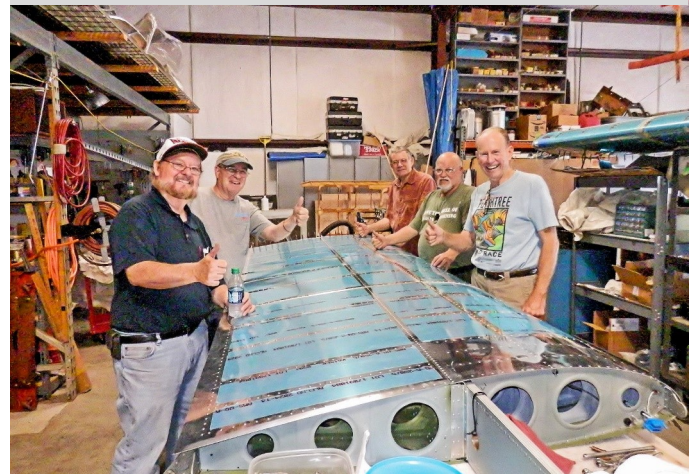
It's thumbs up after pulling that last rivet on the left wing panel, not counting the wing tips that still need work and the flaperons that are next.
