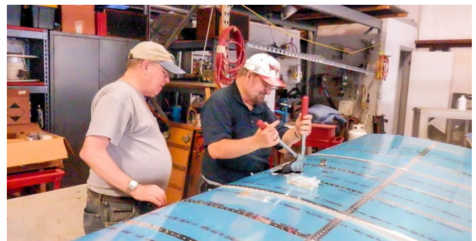
It's thumbs up after pulling that last rivet on the left wing panel, not counting the wing tips that still need work and the flaperons that are next.
