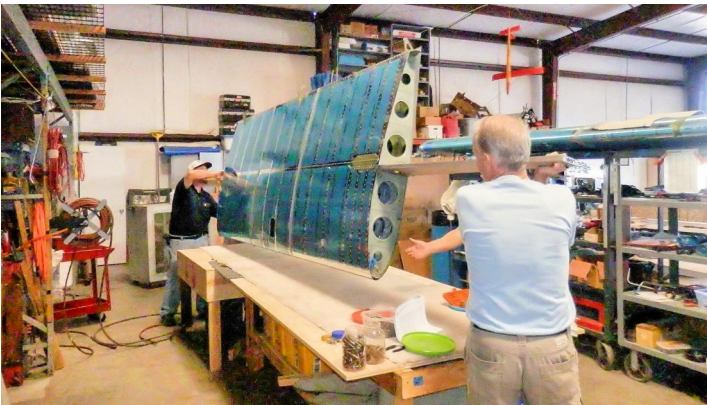
It's thumbs up after pulling that last rivet on the left wing panel, not counting the wing tips that still need work and the flaperons that are next.
